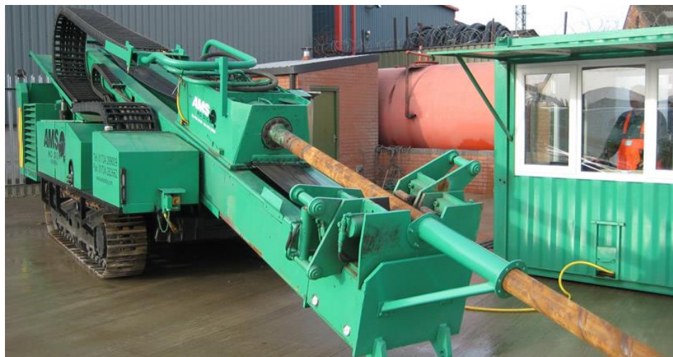
Powerbore 70 tonne directional drilling rig as used at Sizewell
