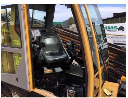
A roomy climate-controlled cab allowing the operator to drill in comfort no matter what the weather conditions. This model also features the joystick controls now common throughout the Navigator line up, saving time and money on future operator training.
